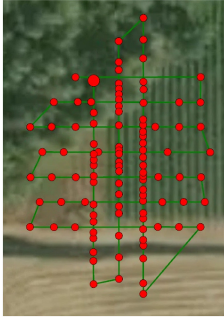
Figure 3.4. UAV flight paths (a) automatic grid flight plan of DJI Mavic 3M, (b) manual setup waypoints path of DJI Mini 4 Pro.
