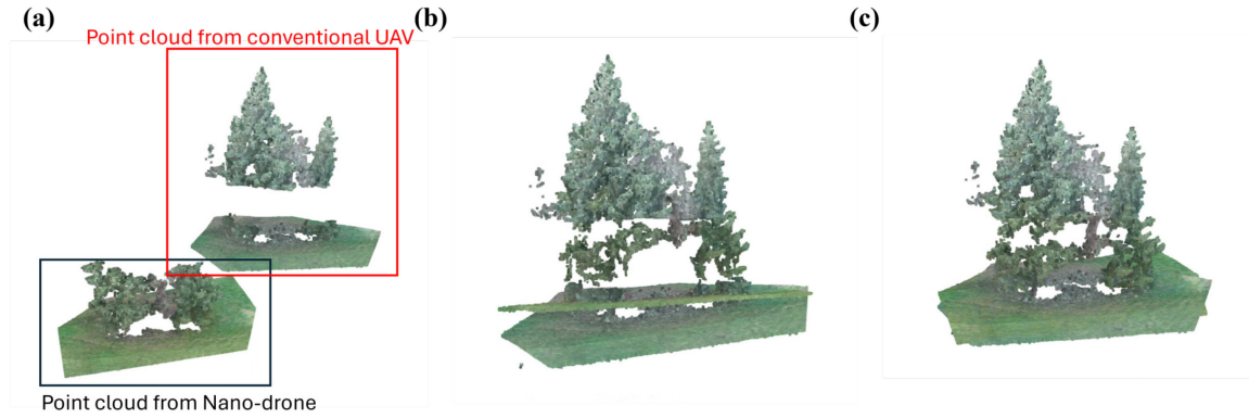
Figure 3.7. Example of point cloud alignment by steps (a) raw point cloud by two sources, (b) integrated point cloud by transformation matrix, (c) integrated point cloud by ICP fine alignment.
