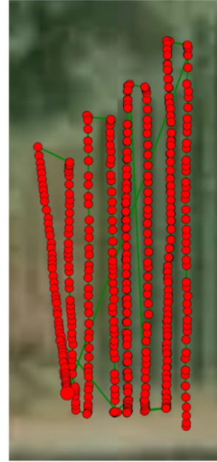
Figure 3.4. UAV flight paths (a) automatic grid flight plan of DJI Mavic 3M, (b) manual setup waypoints path of DJI Mini 4 Pro.
