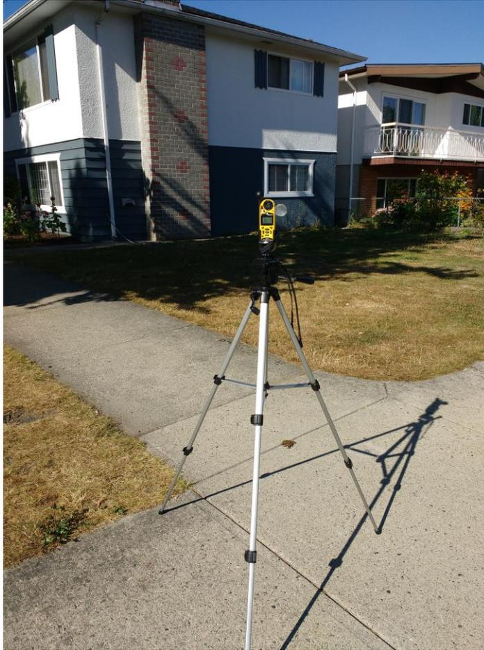
Figure 3-2: Portable heat stress meter (Kestrel 4600) mounted at 1.1 m on a tripod used for the evaluation of simulated  $T_{mrt}$  values.
