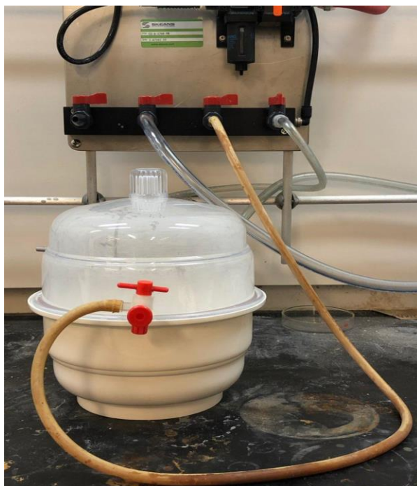
Figure 2.4. Chemical vapor deposition set-up including a vacuum desiccator, connecting tubes and vacuum suction apparatus.
