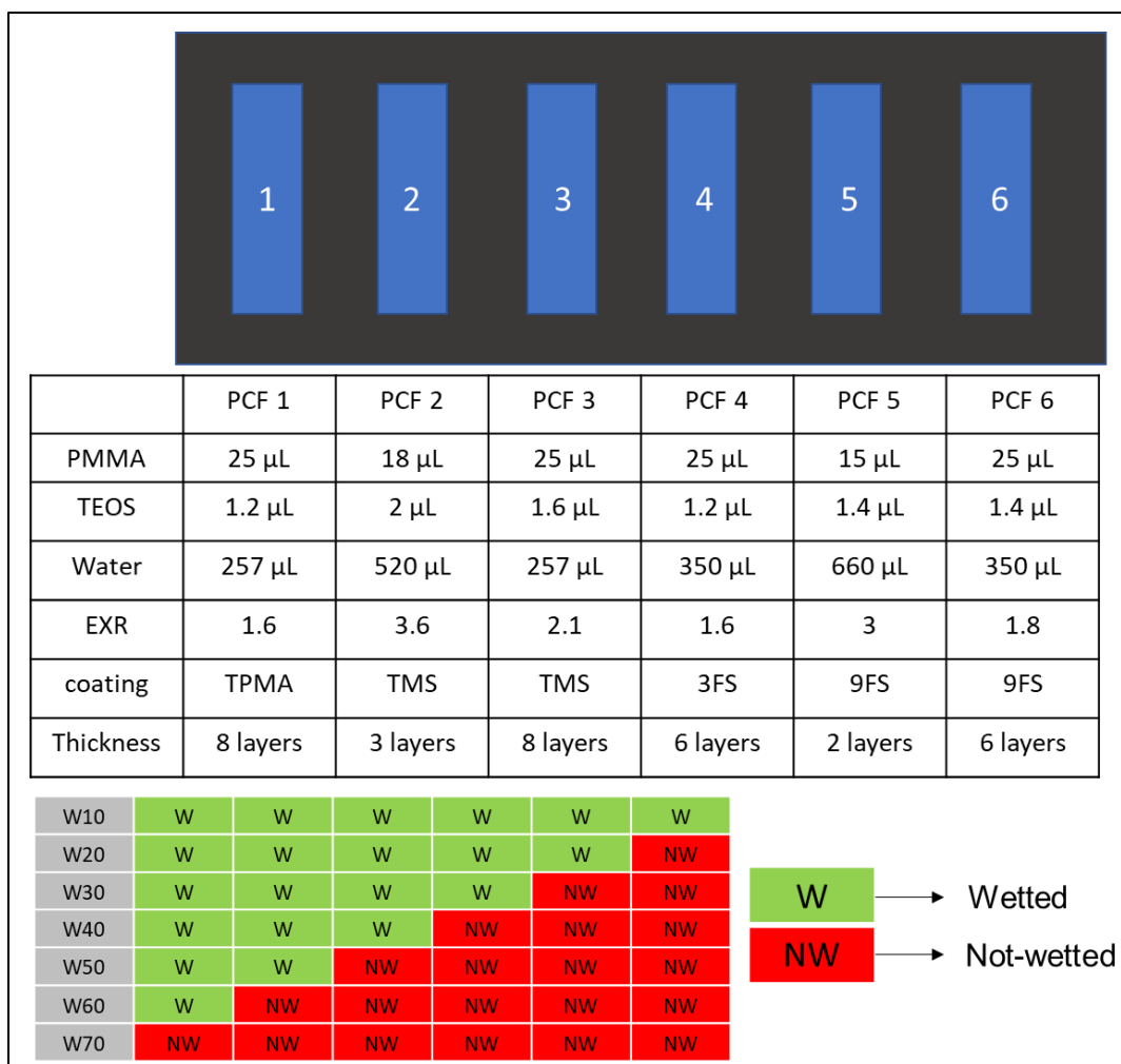
Figure 5.12. Schematic design and composition details of six PCFs on the sensor to differentiate seven different water/EtOH mixtures: W10, W20, W30, W40, W50, W60 and W70.
